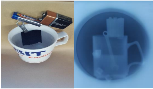
Fig.2 Photograph of a cup filled with water, a mini spanner, and batteries (left), and the fast-neutron imaging by film method in KSTAR tokamak (right).
