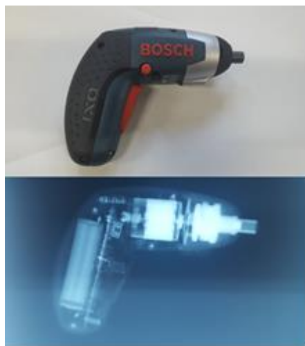
Fig.3 Photograph of a machine drill (upper), and the fast-neutron imaging by film method with the D-D neutron generator (lower).
