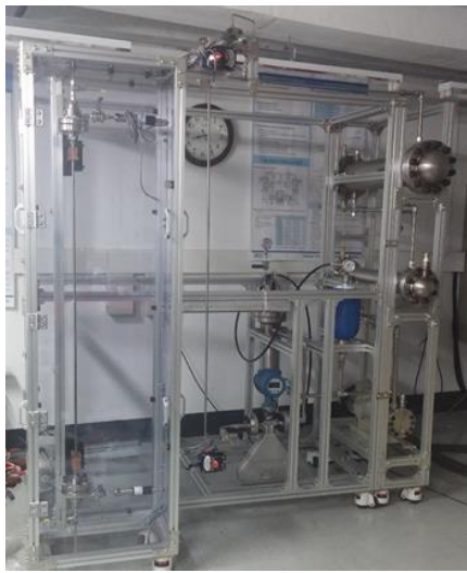
Fig. 5. Pressurized flow boiling loop at THLAB. Major design conditions with the R134a refrigerant are 3.5 MPa in pressure, 120 ^\circ\text{C} in temperature, 50 ^\circ\text{C} in inlet subcooling, and 2000 \text{kg/m}^2\text{-sec} in mass flux.
