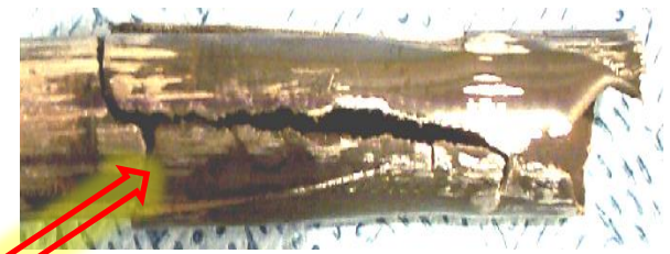
[SCC and Rupture of U-4 SG Tube]
