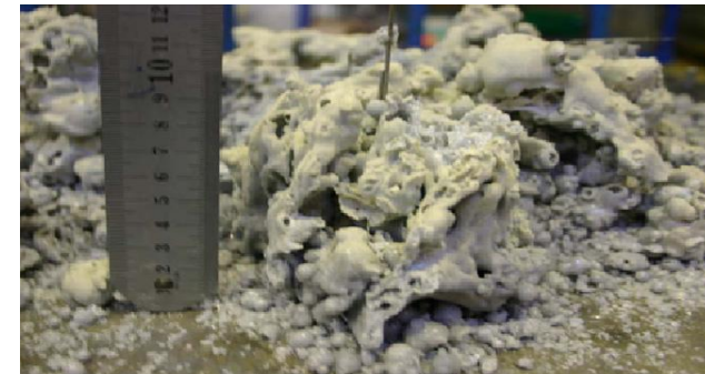
Debris beds formed in DEFOR-E test (Karbojian, A., et al., NED, 2009)
