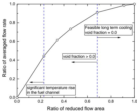
Fig. 4. Effect of the reduced flow area of the recirculation sump on long-term cooling.
