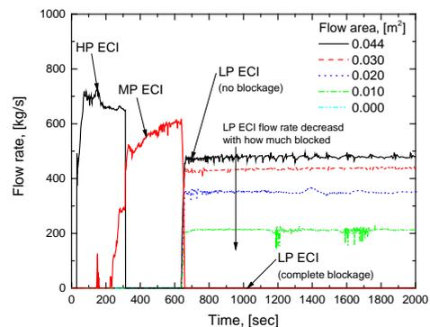
Fig. 2. Variations of ECCS flow rate with the recirculation sump blockage.
