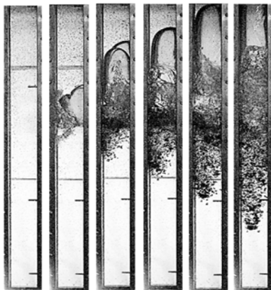
Fig. 2. Fragmentation behavior of melt with 0.18 kg of melt injection mass.
