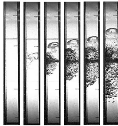
Fig. 4. Fragmentation behavior of melt with 1.40 kg of melt injection mass.
