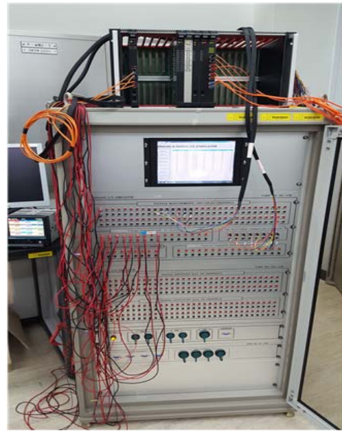
Fig. 4. System Configuration of I/O Stimulator
