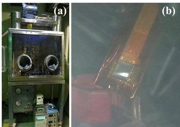
Fig. 3. (a) Glove box in Bank-2 in RIPP, and (b) electroplated Ni-63 onto 99% Ni sheet at current density of 20 mA/cm<sup>2</sup>.
