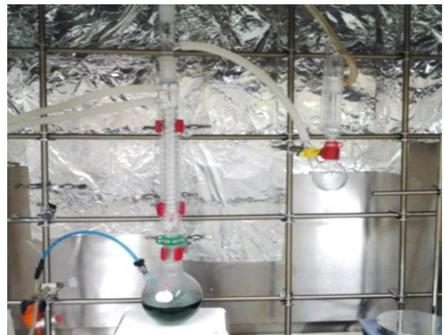
Fig. 2. Dissolution process of irradiated Ni-63 pellets.
