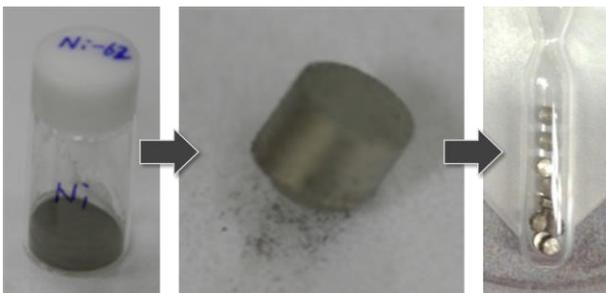
Fig. 1. The pellets of metal Ni-62.
