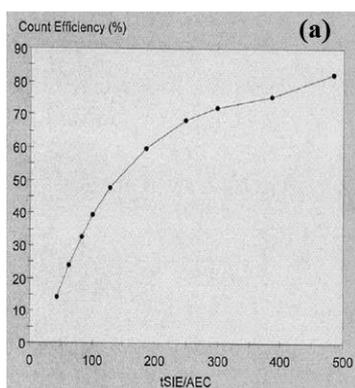
Fig. 4. The quench curve of Ni-63 standard source
