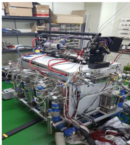
Fig. 1. KIRAMS I-123 Nuclide production system
