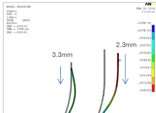
Fig. 9.Maximum displacements in weld region of nozzles
