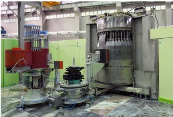
Fig. 1. Cold Neutron Triple-Axis Spectrometer and its modified monochromator shielding at HANARO
