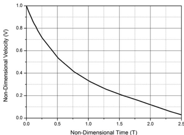
Fig. 4 Analytical coastdown curves for pump #1
