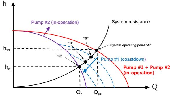
Fig. 3 System H-Q curve during pump #1 coastdown
