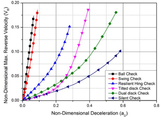
Fig. 2 Dynamic performance of various check valves [1]
