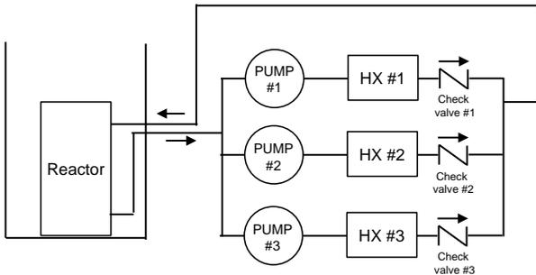
Fig. 1 Schematic diagram of PCS for KJRR
