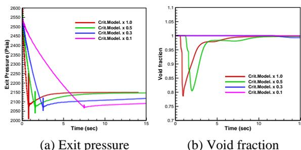
Fig. 5 Profiles of exit pressure and void fraction at POSRV according to the POSRV opening.
