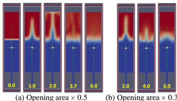
Fig. 4 Void fraction distribution
