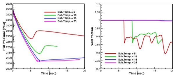
Fig. 3 Profiles of exit pressure and void fraction at POSRV according to the subcooled temperature.
