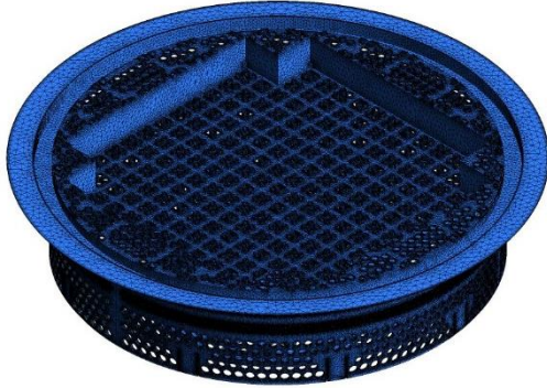
Fig. 3. Grid system; Lower support structure (original LSSBP).
