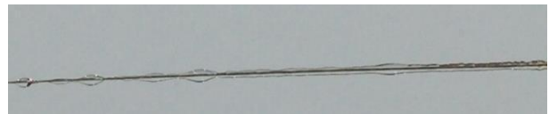
Fig. 4. Deposition layer of CNF on heating wire after the boiling experiments
