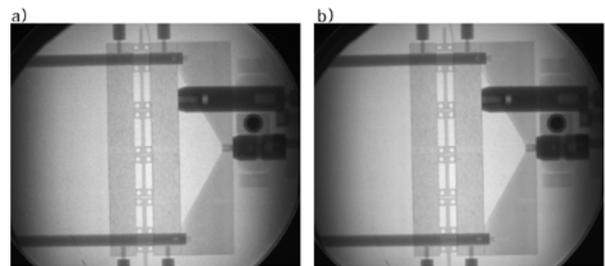
Fig. 2. The effect of median filter; a) Before adjusting median filter, b) After adjusting median filter
