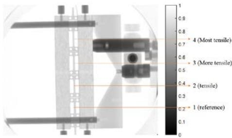
Fig. 3. The corrected image in neutron imaging experiment
