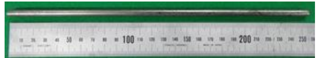
Fig. 1. Typical U-10Zr-10RE fuel slug fabricated with the injection casting process under modest pressure.
