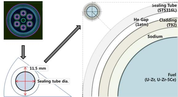
Fig. 1. The cross section of the fuel rod.
