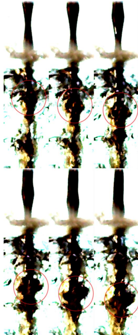
Fig. 1. Post-processed images for formation of mushroom-like shape on the middle of jets by unstable jet injection in MATE 00-2; red circle: boundary layer stripping region
