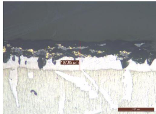
Fig. 7. Cross-section of surface of cladding with SiC<sub>f</sub>/SiC composite protective film of PIP Process after oxidation (1200 °C).
