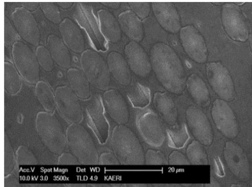
Fig. 9 Surface of CVI SiC<sub>f</sub>/SiC composite after thermal shock test (SEM x3500)
