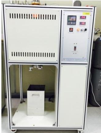
Fig. 4 drop tube furnace for thermal shock test
