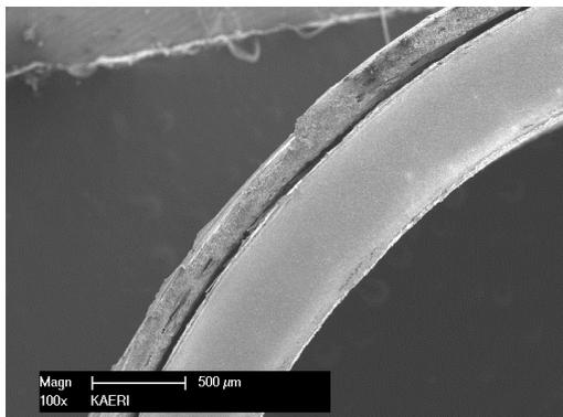
Fig. 8 Surface separation of SiC<sub>f</sub>/SiC composite and Zry-4 after thermal shock test (SEM x100).
