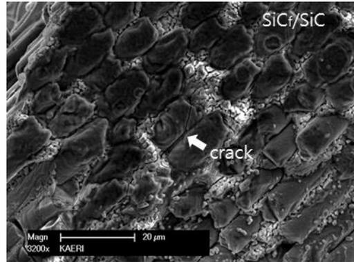
Fig. 9 Surface of PIP SiC<sub>f</sub>/SiC composite after thermal shock test (SEM x3200)
