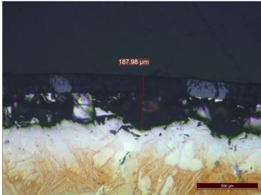
Fig. 7. Cross-section of surface of cladding with SiC<sub>f</sub>/SiC composite protective film of CVI Process after oxidation (1200°C).
