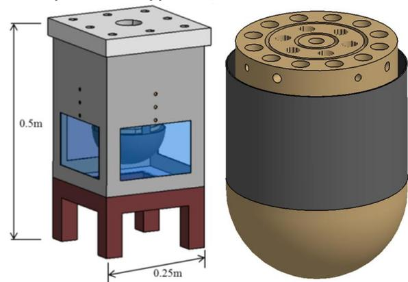
Fig. 1. Schematic of IVR-ERVC experimental apparatus
