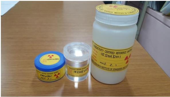
Fig. 2. The photograph of CRMs for measurement efficiency of Gamma Spectroscopy.
