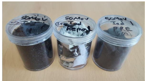
Fig. 1. The photograph of charcoal filter (left), HEPA filter (middle) and pre filter (right) collected in 90 ml plastic containers for sampling.
