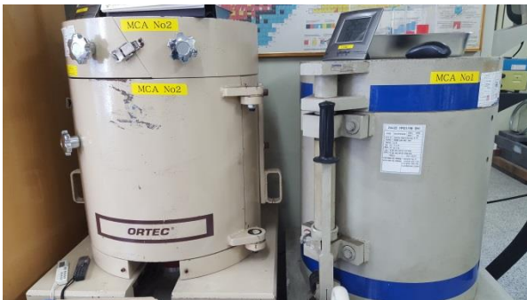
Fig. 3. The photograph of Gamma Spectroscopy to analyze nuclide and radioactive contamination of the used air filters samples.
