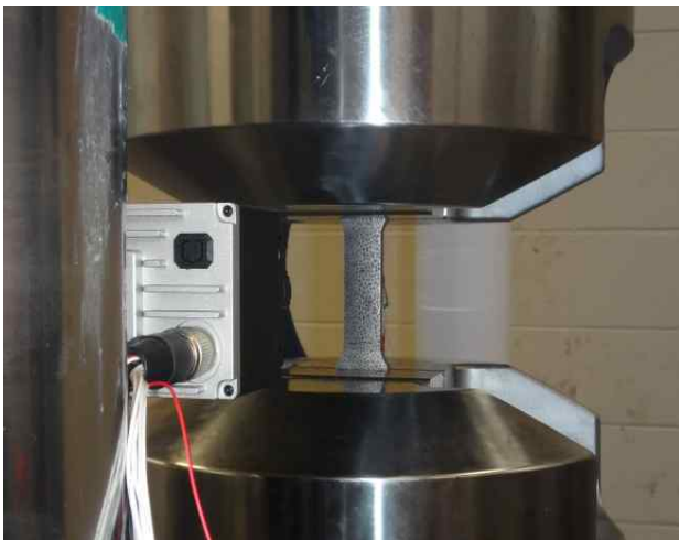
Fig. 4. Specimen and vision-based measurement system
