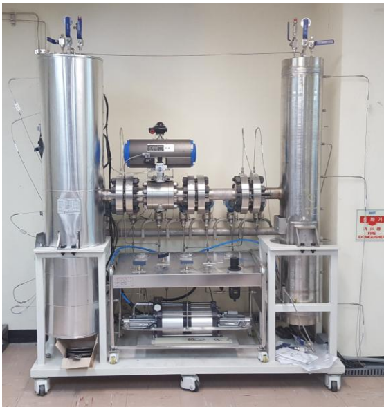
Figure 2 photograph of the experimental facility for CO 2 critical flow test
