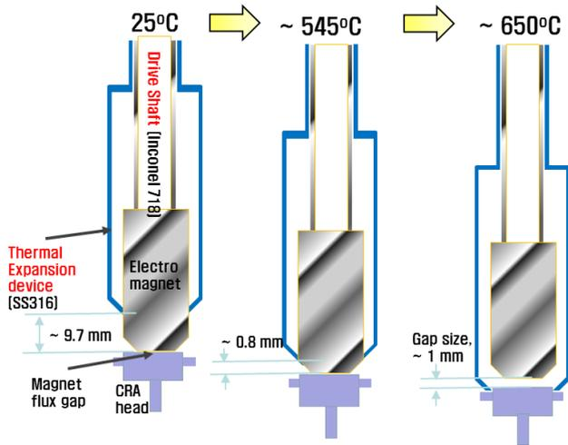
Fig.3 Basic behaviors of thermal expansion device depending on the environment temperature
