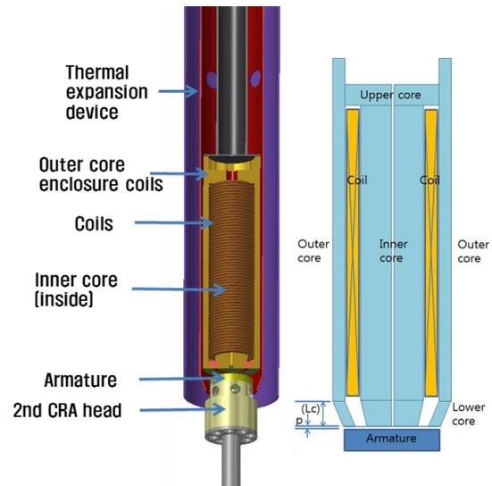
Fig.2 Design concept of electromagnet and thermal expansion device
