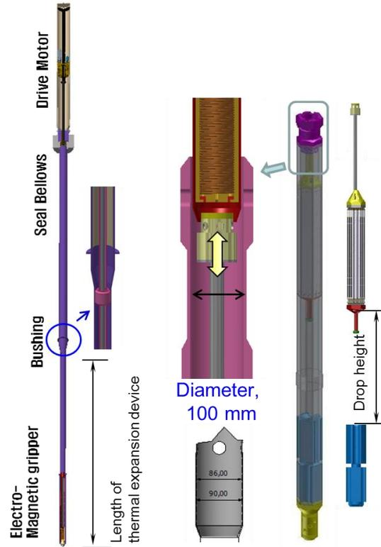
Fig.1 Design concepts of the passive shutdown system and secondary control rod drive system
