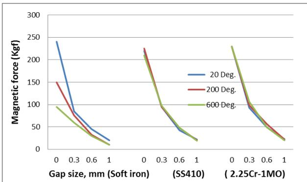
Fig.5 Electromagnetic forces on CRA head of a passive shutdown system
