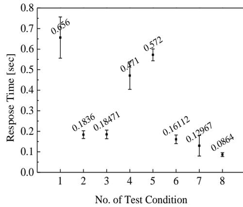
Fig.6 Trigger-off response time of the electromagnet of the secondary control rod drive system
