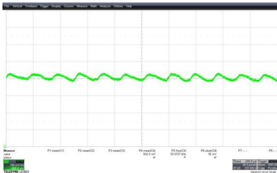
Fig. 4. Measured RF amplitude ripple from DTL
