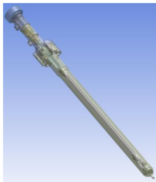
Fig. 2 Three-dimension model of the nuclear test rig in the coolant flow simulator
