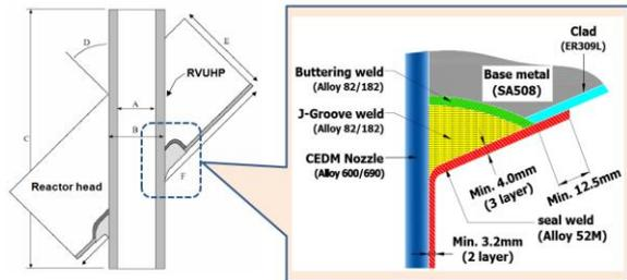
Fig. 2. EFR welding concept for CEDM nozzle
