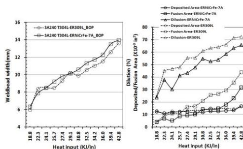
Fig. 5. Comparison on welding results obtained at welding of base metal (SA240 T304L) and different filler wires
