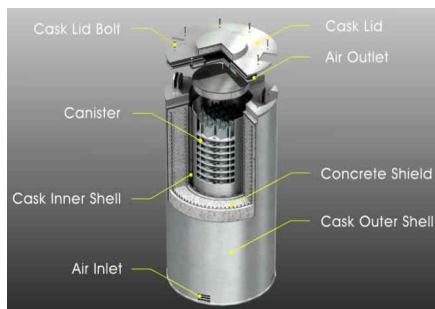
Fig. 1. Configuration of concrete storage cask.
