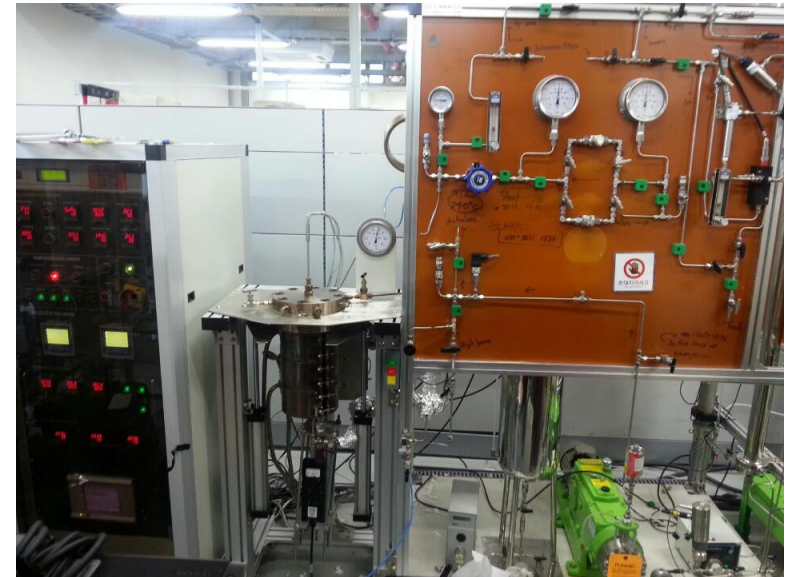
Fig. 7 Oxidation system which can simulate primary water chemistry of nuclear power plant
