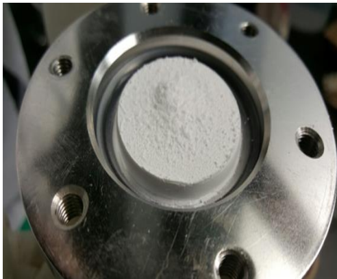
Fig.2: The Aerosol Cake Collected on Glass Fiber Membrane Filter on MTA-3.
