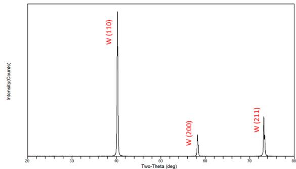
Fig. 1. XRD patterns of the reduced W/TiC powder.
