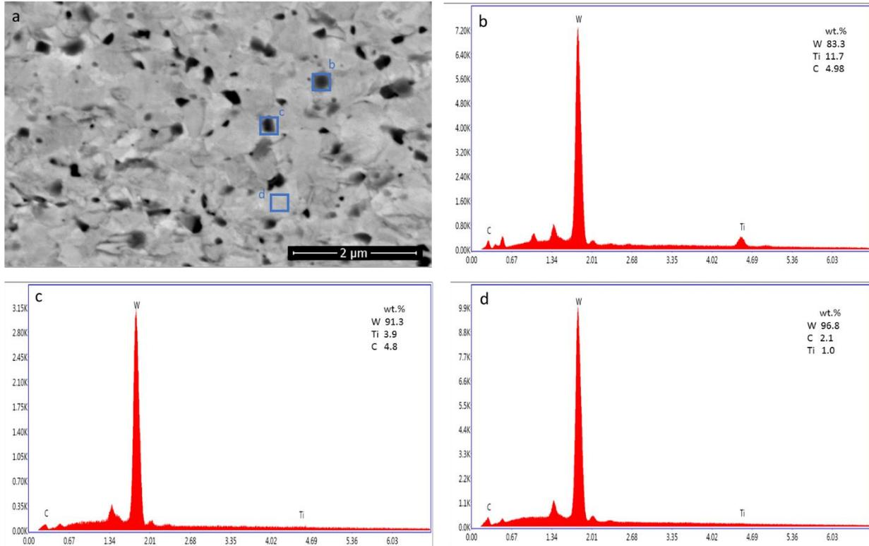
Fig. 2. (a) FESEM image of the sintered W/TiC; (b), (c) and (d) EDS spectrum of the selected square regions.
