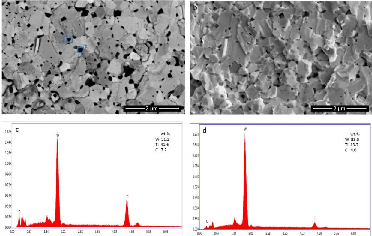
**Fig. 3.** (a) Back scattered electron image (b) secondary electron of the fracture surface sintered W/TiC; (c) and (d) EDS spectra of the selected square regions
