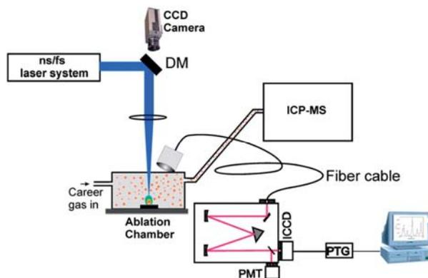
Figure 2. Schematic of LA-ICP-MS [8]
