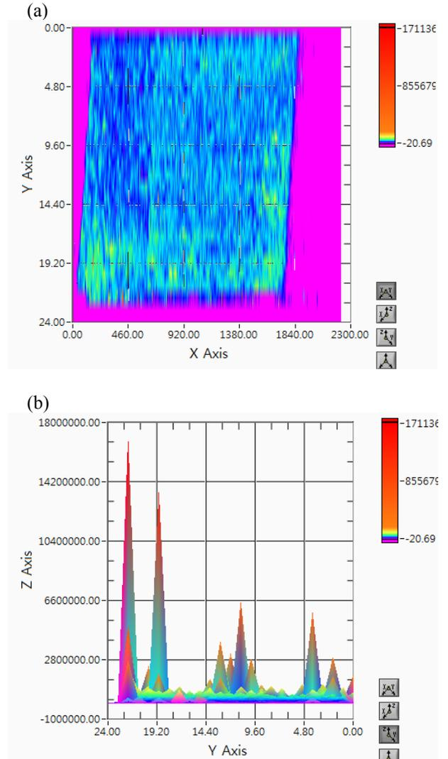
Figure 5. Mapping results (a) X axis (Axial direction) versus Y axis (Radial direction) and (b) Y axis (Radial direction) versus Z axis (Intensity) by using IG-110 Japan lot 1 (99hr)
