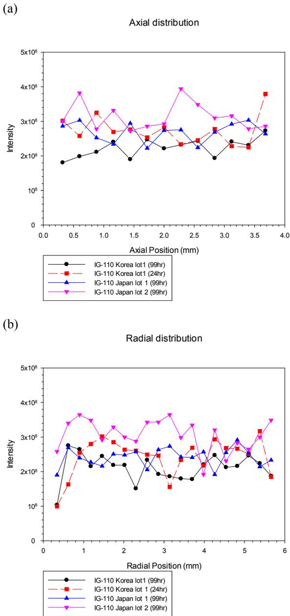
Figure 4. (a) Axial and (b) radial Cs distribution in the sample
