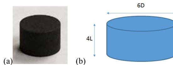
Figure 1. (a) The picture of IG-110 specimen and (b) schematic of specimen
