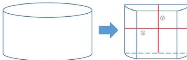
Figure 3. Cutting method for making LA-ICP-MS sample
