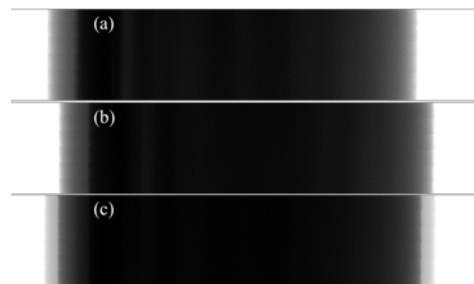
Fig. 7. Projection data from x-ray tube position at (a) 0degree, (b) 3degree, (c) Combined data(Virtually from dual sources).
