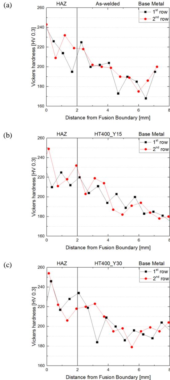
Figure 3. Vickers hardness result from the fusion boundary between Alloy 182 and Alloy 600 to the Alloy 600 base metal. Each graph shows the result of (a) as-welded, (b) HT400\_Y15, and (c) HT400\_Y30 case respectively.
