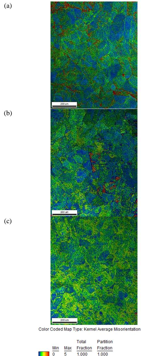
Figure 5. KAM mapping on Alloy 600 HAZ distance from the fusion boundary about 700µm. Above three pictures show KAM distribution of (a) as-welded, (b) HT400\_Y15, and (c) HT400\_Y30 specimens.
