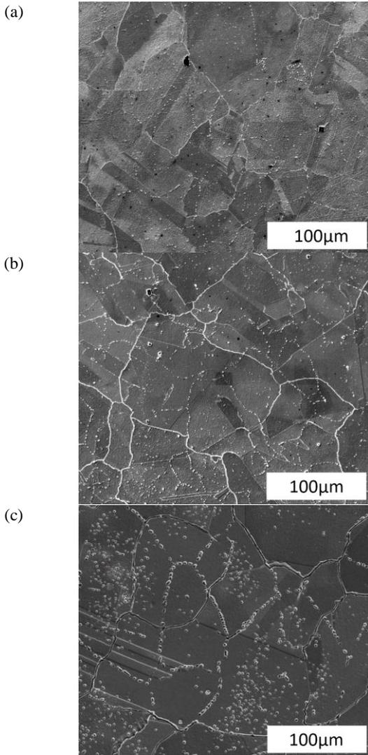
Figure 4. Distribution of Cr precipitates on the surface of (a) as-welded, (b) HT400\_Y15, and (c) HT400\_Y30 specimen respectively pictured by scanning electron microscopy (SEM).
