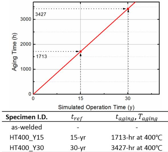
Figure 2. Aging time at the temperature 400°C to simulate 15 years and 30 years at the temperature 320°C in nuclear power plant respectively.
