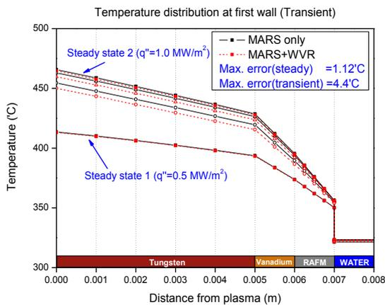
Fig. 6. Comparison results between MARS code and first wall module coupled with MARS DLL
