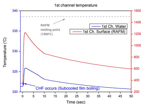
Fig. 9. 1<sup>st</sup> channel surface and coolant temperature
