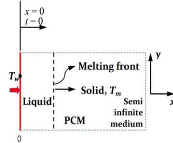
Fig. 4. One-dimensional Stefan's problem for semi-infinite medium [8]
