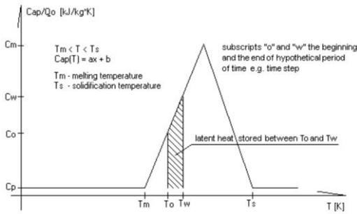
Fig. 3. Graphical representation of effective heat capacity method [7]
