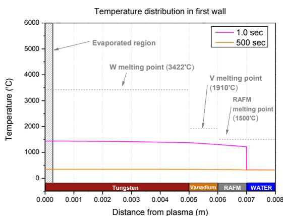
Fig. 8. Temperature distribution in first wall (1.0 ~ 500 sec)
