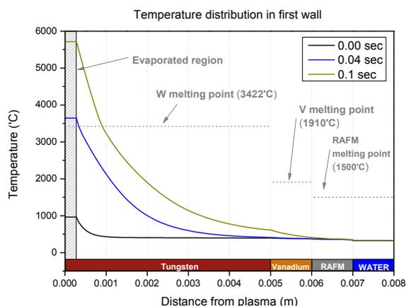
Fig. 7. Temperature distribution in first wall (0.0 ~ 0.1 sec)
