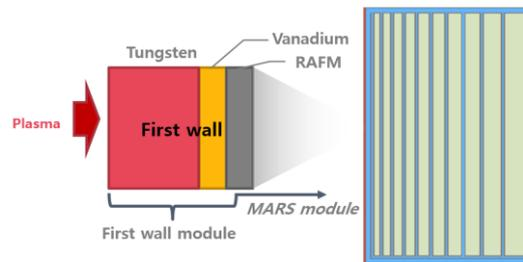
Fig. 1. Modeling range of first wall module and MARS code in a single blanket module
