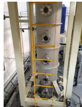
Fig. 3. High pressure test loop for single scrubbing nozzle.
