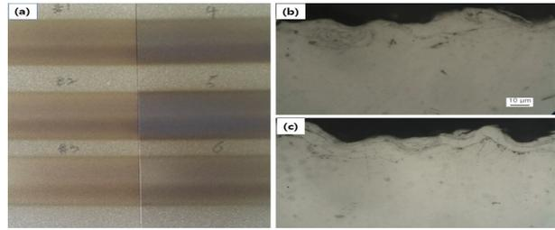
Fig. 4. cold spray processed ODS layer. (a) optical micrograph from the plane view. (b) scanning electron micrograph from the cross section view.
