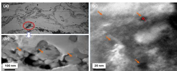
Fig. 3. (a) Heat affected zone in the coated ODS layer (b)  $\text{Cr}_2\text{O}_3$  phases (c)  $\text{Y}_2\text{Ti}_2\text{O}_7$  nano particles.
