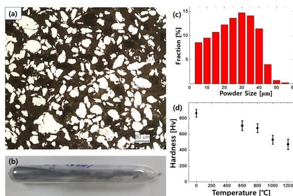
Fig. 1. (a) Mechanically Alloyed powder of ODS for the spray process. (b) Quartz tube for heat-treatment of powders. (c) Size distribution of mechanically alloyed
