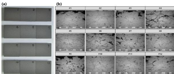
Fig. 2. Images of HVOF processed ODS layer. (a) optical micrograph from the plane view. (b) scanning electron micrograph from the cross section view
