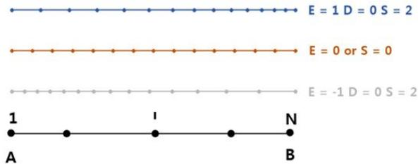
Fig. 2. Example of point distribution for each E, D, S case
