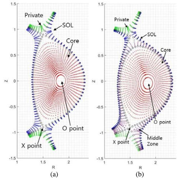
Fig. 3. Test grid applied for KSTAR (a) CDN case, (b) DDN case
