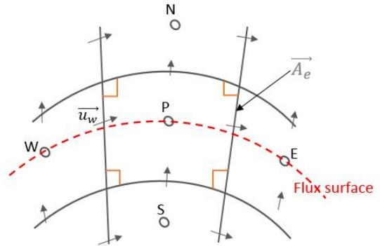
Fig. 1. Schematic cartoon for a control volume of FVM
