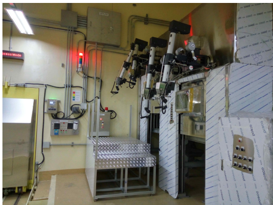
Figure 2. Hot-Cell constructed in PR101 of KOMAC for the treatment of irradiated targets.
