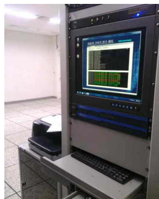
Figure 3. Centralized RMS data server
