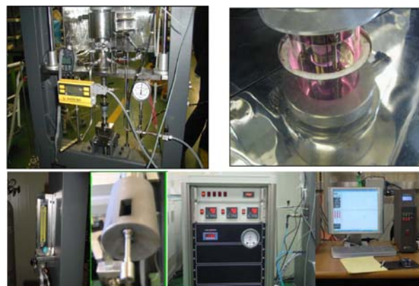
Fig. 1. Creep testing apparatus of He environment installed at KAERI.
