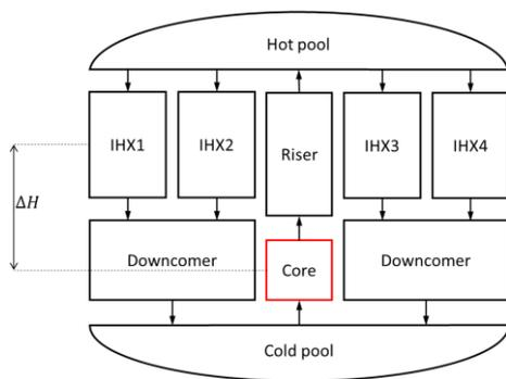
Fig. 1. Schematics of the primary loop of the AHR400
