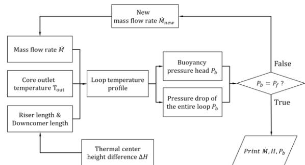
Fig. 2. Calculation algorithm of the analysis using the MATLAB
