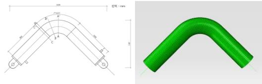
Fig. 1. Test specimen and FE model of elbow
