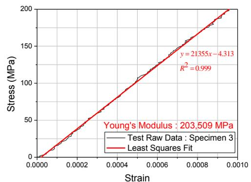
Fig. 2. Estimation of modulus of elasticity
