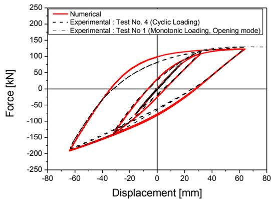
Fig. 4. Result comparison between numerical analysis and test under cyclic loading
