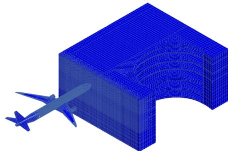
Fig. 2. Finite element model of and nuclear structure
