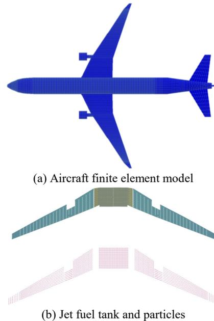
Fig. 1. The modeling of aircraft and jet fuel
