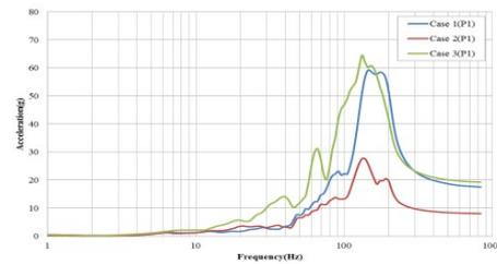
Fig. 7. Floor response spectrum for the impact velocity (50, 100, 150m/s) at P1
