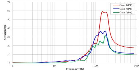
Fig. 6. Floor response spectrum for the impact velocity (50, 100, 150m/s) at P1
