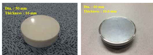
(a) RbCl pellet and its target cladding
