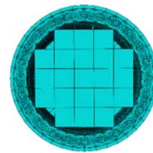
Fig. 2. FEM model of 21 fuel assemblies inside the cask
