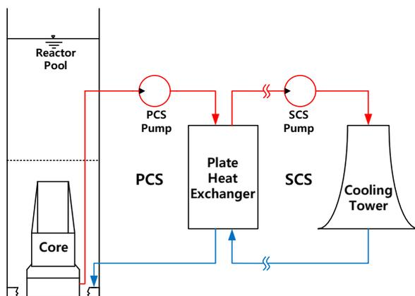
Fig. 1. Schematic diagram of system.
