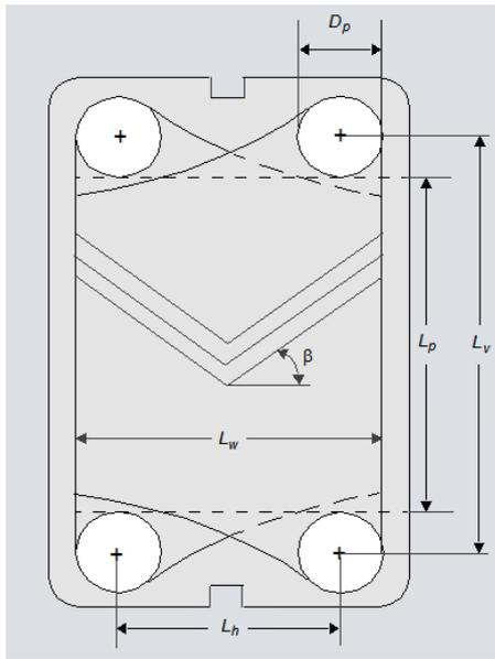
Fig. 3. Geometry of PHE.
