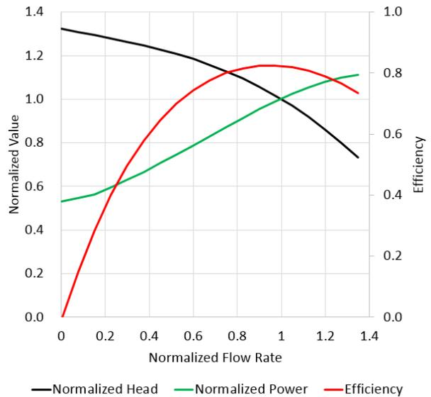
Fig. 4. Pump performance curve
