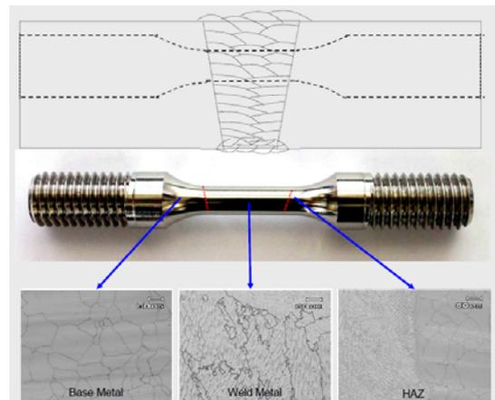
Fig. 1. Schematic diagram showing cutting of specimen with respect to GTAW welded plate, and the microstructures.
