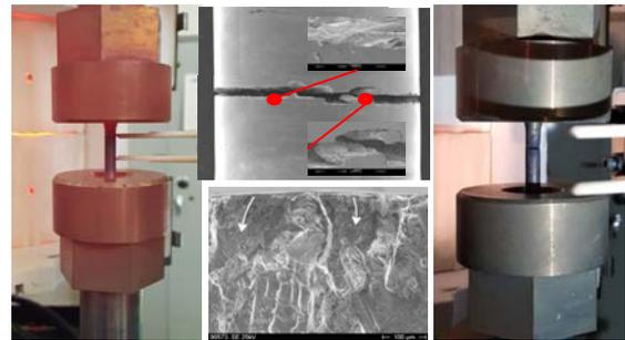
Fig. 5. Failure photographs and SEM after LCF testing.
