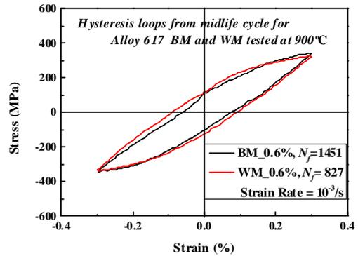
Fig. 4. Hysteresis loops for BM and WM specimens.
