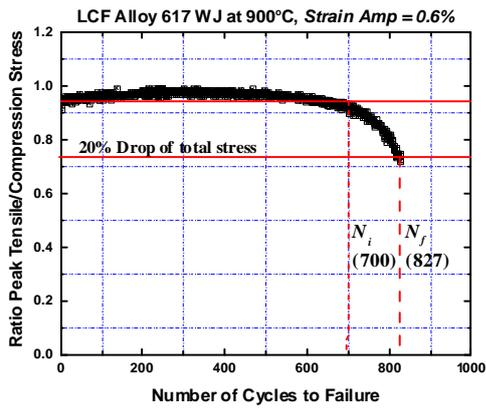
Fig. 2. Illustration of LCF failure criterion for BM specimen.
