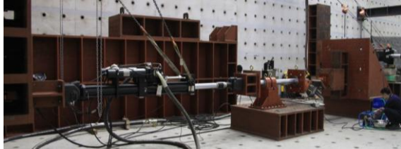
Fig. 4. Dynamic test setup configuration using straight moving zig, hinge elements, and elbow specimen.
