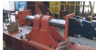
Fig. 2. A special zig to ensure the straight movement of actuator.
