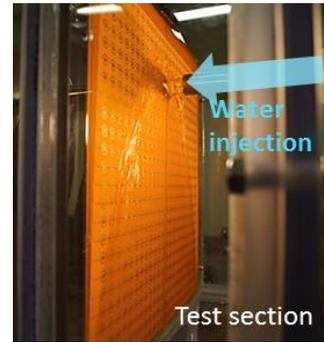
Fig. 10. FPCB Liquid film sensor and downward liquid film flow of the experiment
